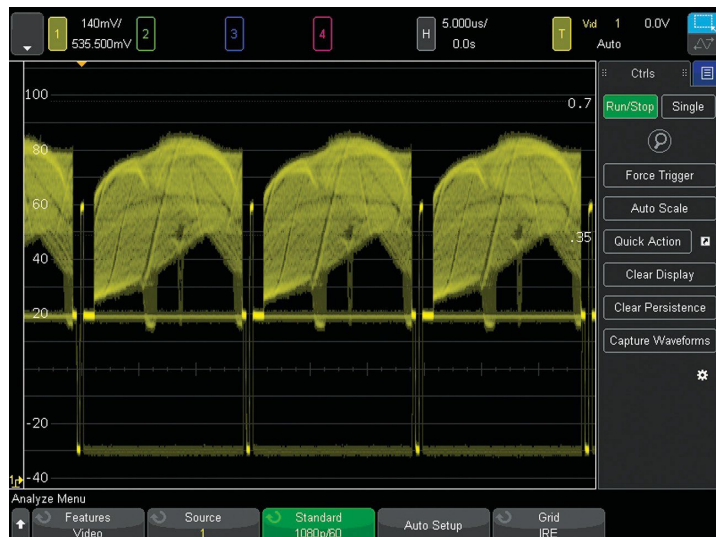
Figure 27. Triggering on 1080p HDTV signal analysis.
