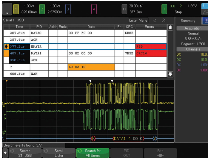
Figure 21. USB 2.0 trigger, decode and "lister" display.
