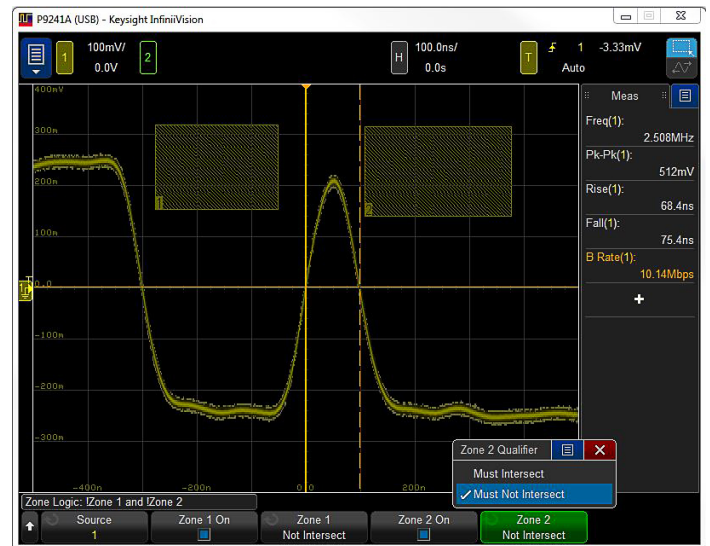
Zone Trigger enable quick and easy isolation of the data pattern of interest.
