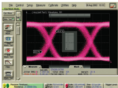
Characteristic optical unfiltered eye measurement (86116C-041).
