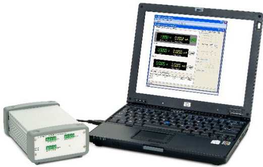
Figure 1. U2722/3A used as a standalone instrument
